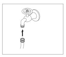
**STEP 2:** Attach high pressure hose between pressure washer and machine. Turn garden hose water on. Additional adapters and couplers may be needed to connect your brand of pressure washer to the machine.
